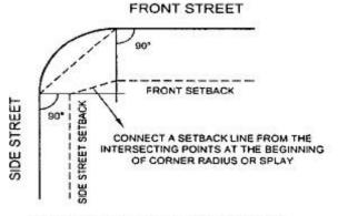
METHOD FOR ESTABLISHING THE BUILDING SETBACK AT STREET CORNERS Unless noted on the plan. The minimum front setback on a splayed or curved street frontage must be taken in an arc connecting the front street setback line to the side street setback line commencing at the points that are perpendicular to the points where the street alignment commences to arc.
