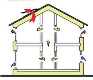
Stack effect ventilation through openable glazing
