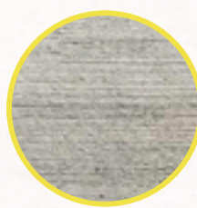
GENERAL FOOTPATHS Insitu Grey concrete, light broom finish (without picture-framed edges)
