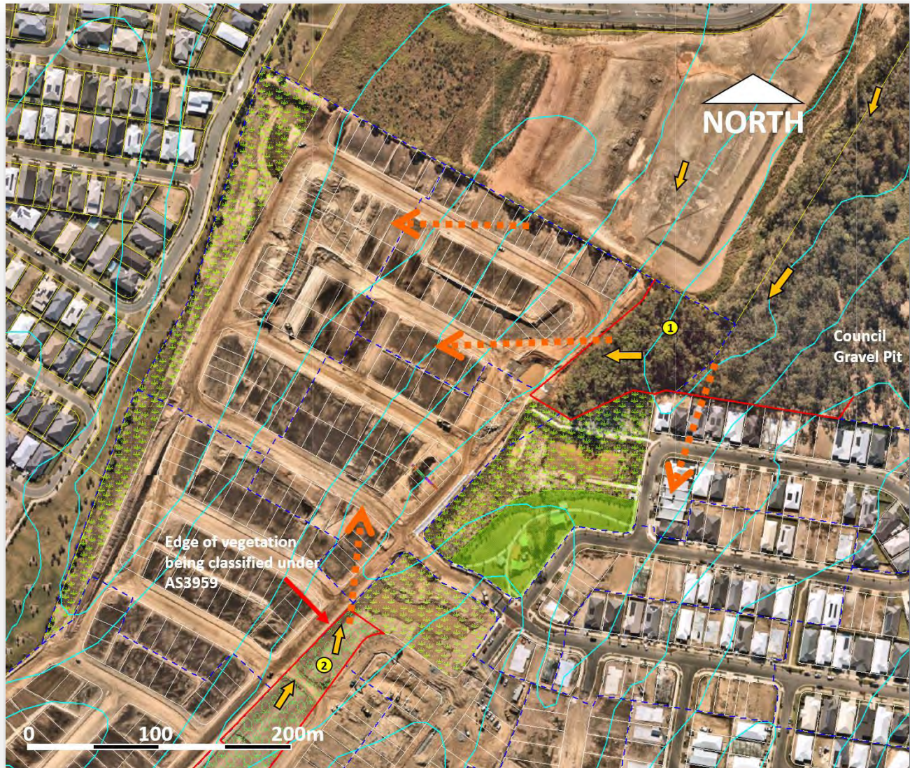
Figure 4. Fuel accumulation, slopes and setback. Solid arrows show most likely direction of bushfire attack.
