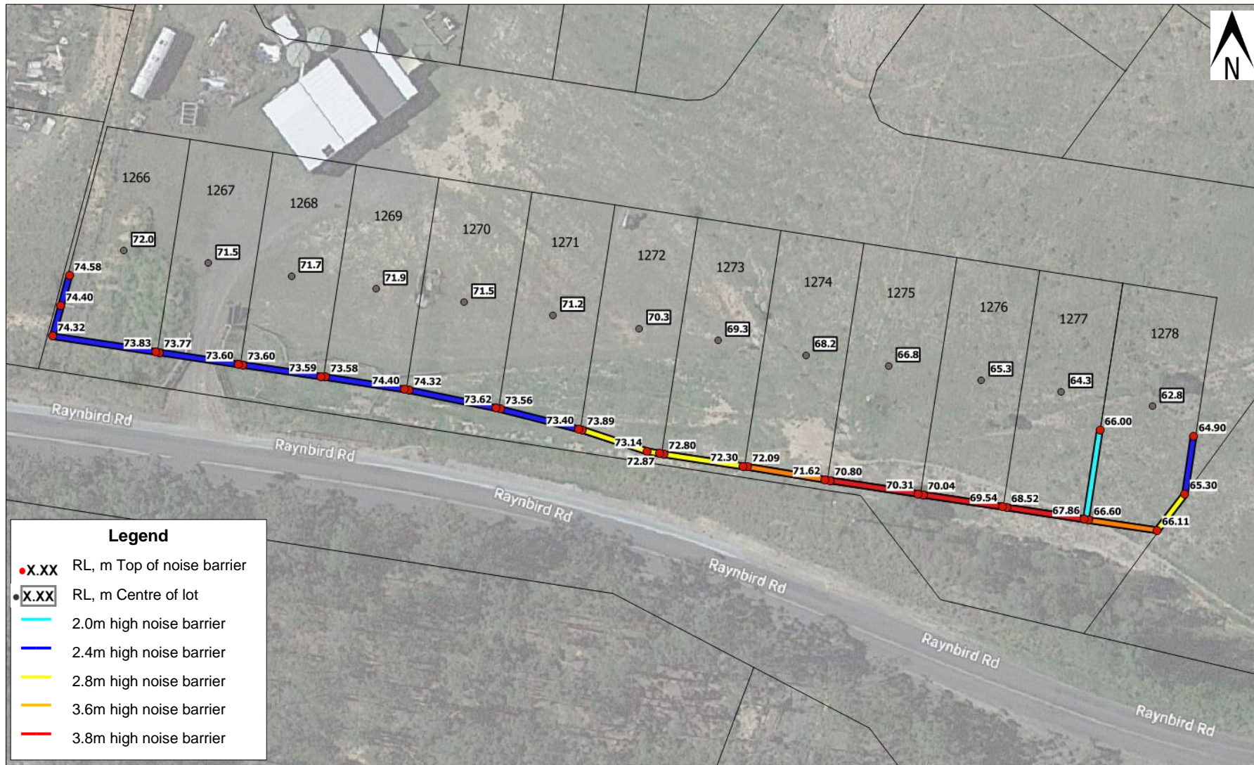
Figure 6.1 Noise Barrier Alignment – Stage 12
