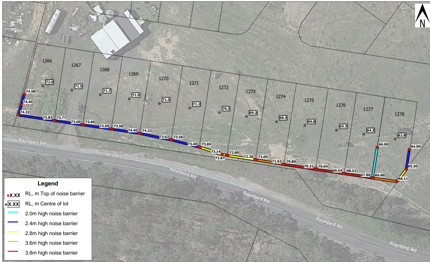
Figure 6.1 Noise Barrier Alignment – Stage 12
